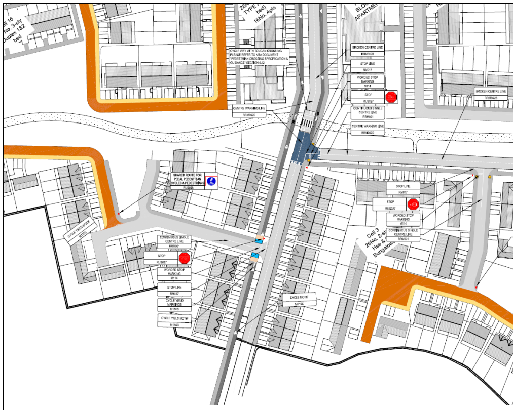
Figure 4.2: Proposed Street Linking Permitted Phase 1a and Proposed Phase 1b Developments (Source: JOR Drawing Road Signage & Markings Layout Plan Sheet 2 of 3, ref. 033, rev. 3)
